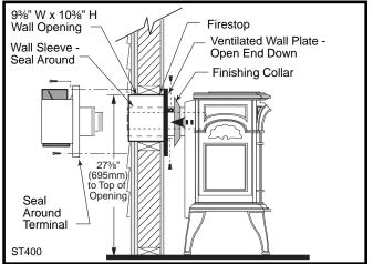
Fig. 18 SDVR with Rear Vent Kit 7TFSRSK installation.
